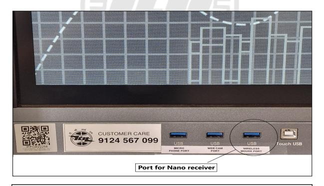
The Port with the "Wireless Mouse Port" mentioned is to be used to connect the Nano receiver of the keyboard and mouse.
