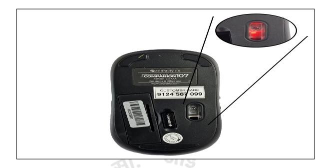
• If there is no red light indication, check the batteries and replace them with fresh ones if necessary, ensuring the correct polarity.
