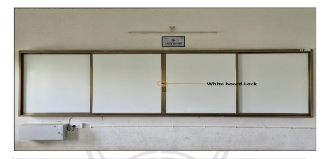
The sliding white board comes with a lock to protect the things under it, such as the IFP Panel, Router, Microphone Receiver, and Web Camera
