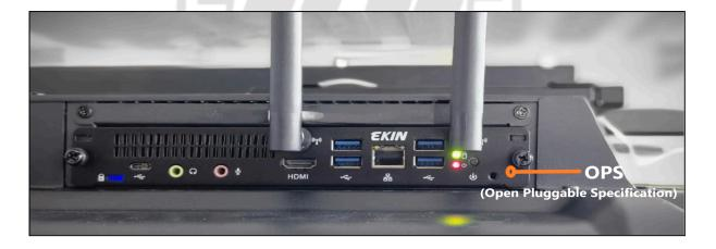
The OPS is placed behind the IFP Display in the assigned slot, and it turns on by itself once the IFP is turned ON.
